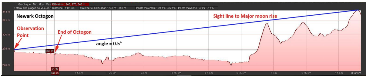
Figure 2. The altitude angle of major moonrise scene from the observation point. The diagram is exaggerated to facilitate understanding. (profile Google Earth)
