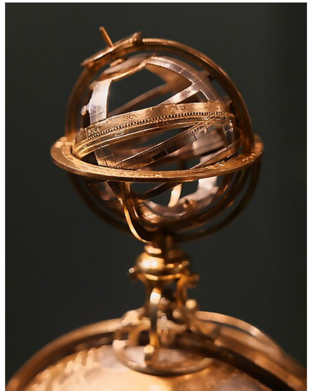
A historical armillary sphere in the Historical Museum of Basel (Switzerland) with three movable rings that describe the three astronomical planes of the horizon, the celestial equator and the ecliptic. Even the ancient Babylonians observed events in the night sky with simple designs of such armillary spheres.
