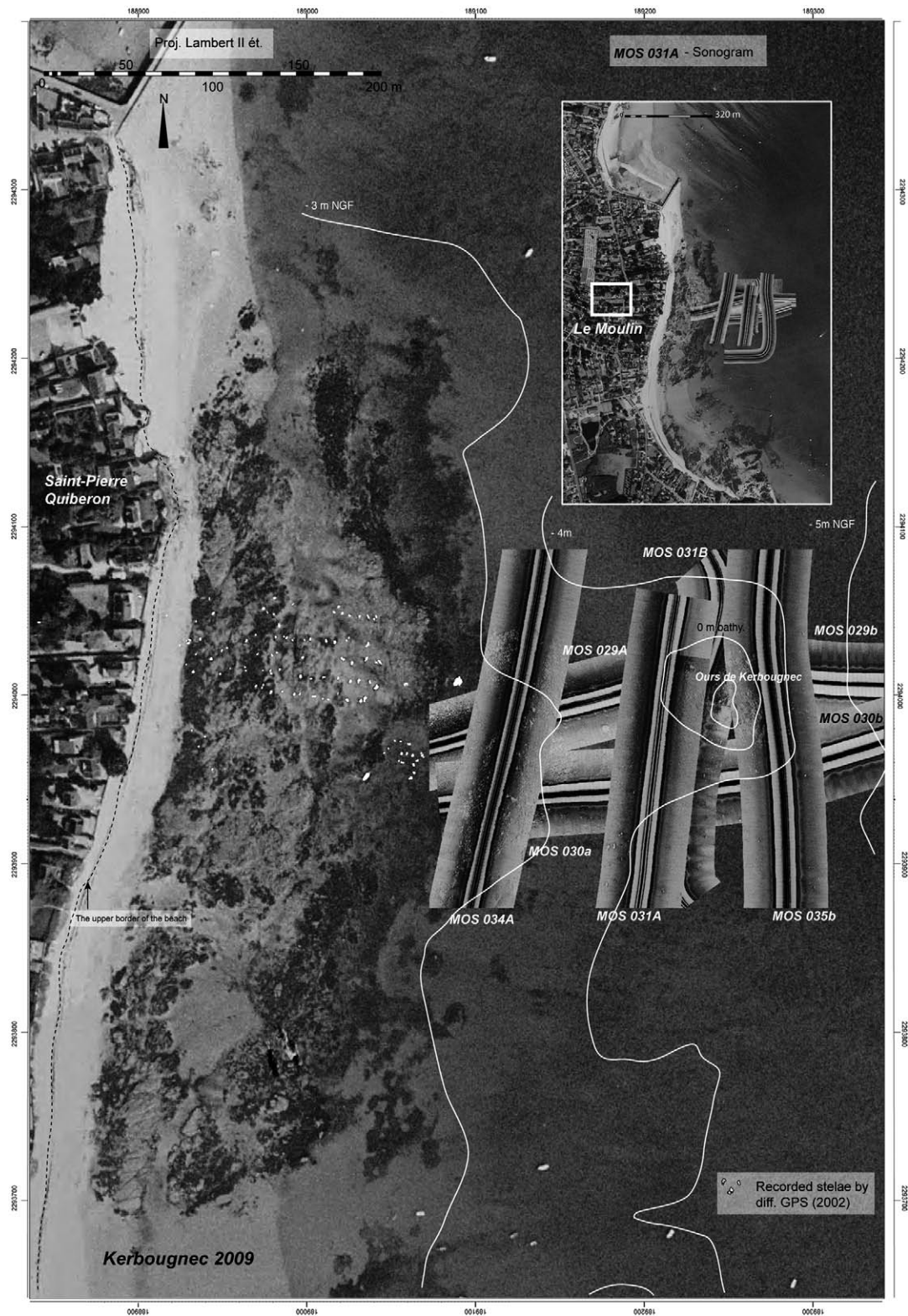
Figure 9.6: Kerbougne. Side-scan sonogram mosaic between the rocky intertidal platform and the Ours shoal (Photo: IGN 2000)
